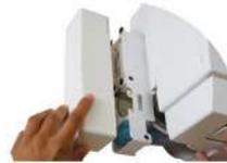
Access to the pump elements (reservoir, tubes etc.) is made by removing the cover.
